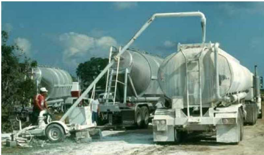
Figure 7: Jet slurry mixer
