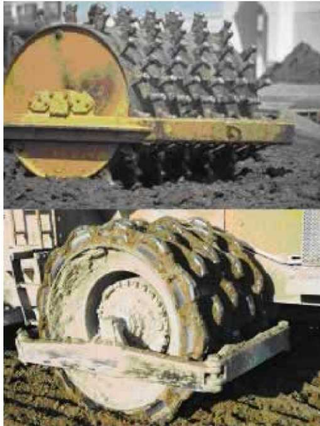
Figure 17: Sheepsfoot (above) & padfoot (below) rollers
